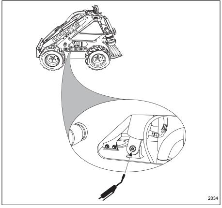
Figure 3-5 Loader Arm Lift Cylinder Base Lubrication Point
